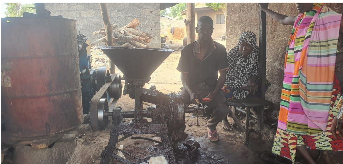
Photo from Aaaie community in Niger State community; shea butter grinding machine powered by 6 horsepower lister engine type machine. Source – Happy Amos (2 July 2023)
