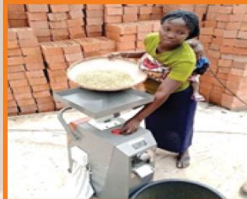
Rice threshing and polishing machine used at Nayo Tropical Technology Mini-grid Kilankwa site Gwagwalada
