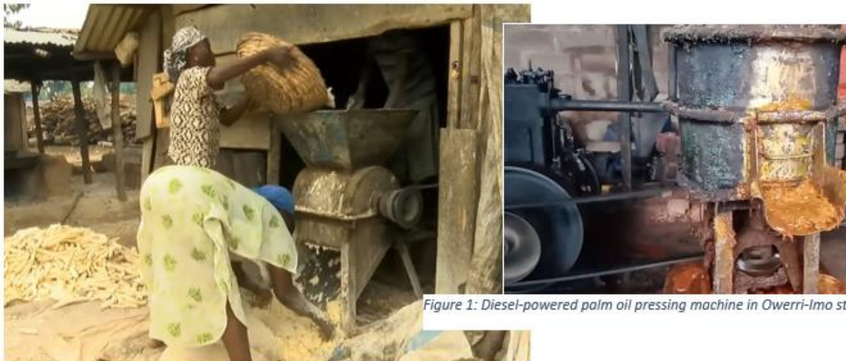
Figure 2: 8-horse power diesel engine cassava girding machine in Ajegunle, Oyo East, Ibadan.
